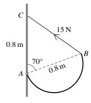
A uniform wire has the shape of a semicircular arc, with diameter AB of length 0.8 m. The wire is attached to a vertical wall by a smooth hinge at A. The wire is held in equilibrium with AB inclined at  $70^{\circ}$  to the upward vertical by a light string attached to B. The other end of the string is attached to the point C on the wall 0.8 m vertically above A. The tension in the string is 15 N (see diagram).
